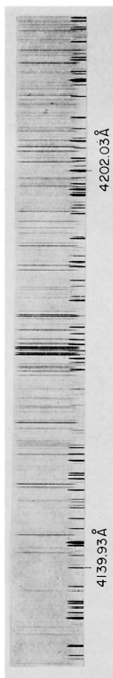
Figure 16 Emission band observed in a discharge through \text{H}_2\text{S} and probably due to \text{H}_2\text{S}^-
